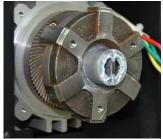
Step 8 -remove the shear key
