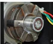
Step 7 –remove the bearing cover
